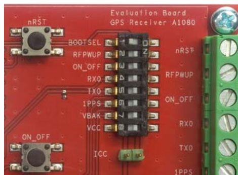
Figure 7: DIP Switches with default settings (SW3)
